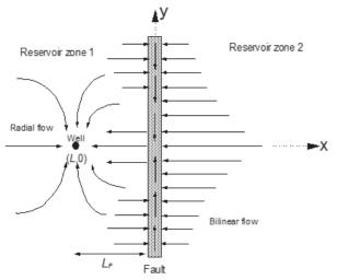
Figure 1.Schematic a finite-conductivity fault displaying the streamlines, after Anisur Raman et al. [11]
