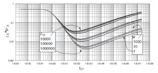
**Figure 2.** Effect of mobility ratio on pressure derivative dimensionless.  $s_F = 0$  y M > 1
