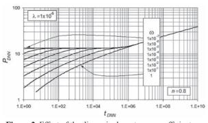
Figure 2. Effect of the dimensionless storage coefficient on the pressure response of a heterogeneous reservoir
