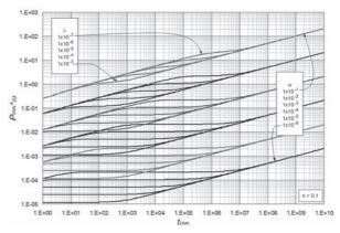
**Figure 7.** Effect of  $\lambda$  and  $\omega$  on the pressure response for a dual-porosity reservoir, n = 0.1
