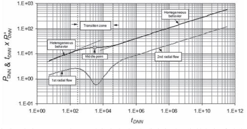
Figure 1. Dimensionless pressure and pressure derivative log-log plot displaying the typical behavior of a dual-porosity reservoir for  $\omega$ =0.01,  $\lambda$ =1x10-7 and n=0.25
