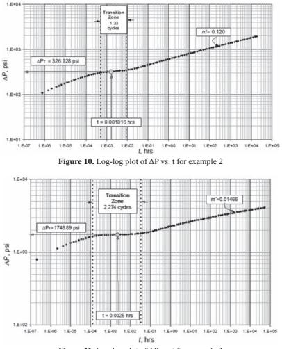
**Figure 11.** Log-log plot of  $\Delta P$  vs. t for example 3
