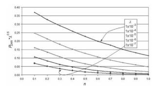
**Figure 5.** Effect of the interporosity flow parameter on the dimensionless pressure multiplied by the square root of the interporosity flow parameter versus the flow behavior index.
