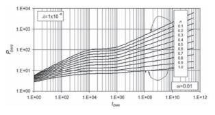
Figure 4. Effect of flow behavior index on pressure response in a heterogeneous reservoir
