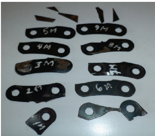
Figure 7. Cushioning plate from clutch disc.
