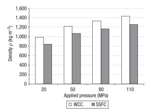
Figure 3. Average density values (kg  $m^{-3}$ ) of WCC and SSFC obtained using different pressure levels (20, 50, 80 and 110 MPa).
