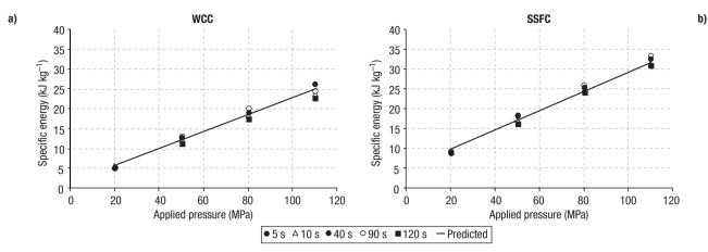
Figure 4. Relationship between applied pressure and specific compression energy to form the WCC (a) and SSFC (b) briquettes (pressure range 20-110 MPa).
