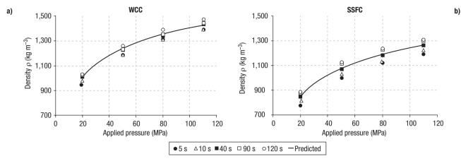
Figure 2. Effect of pressure and pressure application time on the density of WCC (a) and SSFC (b).
