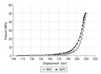
**Figure 6.** Force-displacement plot comparison between SSFC and WCC obtained applying 50 MPa for 40 s.
