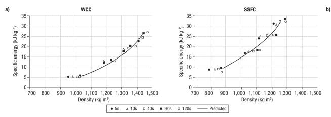
Figure 7. Relationship between specific compression energy and density to form the WCC (a) and SSFC (b) briquettes.
