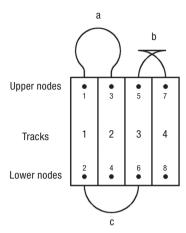
Figure 1. Representation of tracks, their nodes, and prevalent types of headland turnings: (a)  $\Omega$ -turn, (b) T-turn, (c) Π-turn.
