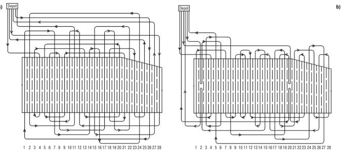
**Figure 5.** Harvest pattern suggested by the operators for covering field B: (a)  $\sigma^{\exp 1}$ , and (b)  $\sigma^{\exp 2}$ .
