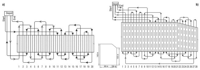
Figure 2. B-patterns generated for covering: (a) Field A, and (b) Field B.
