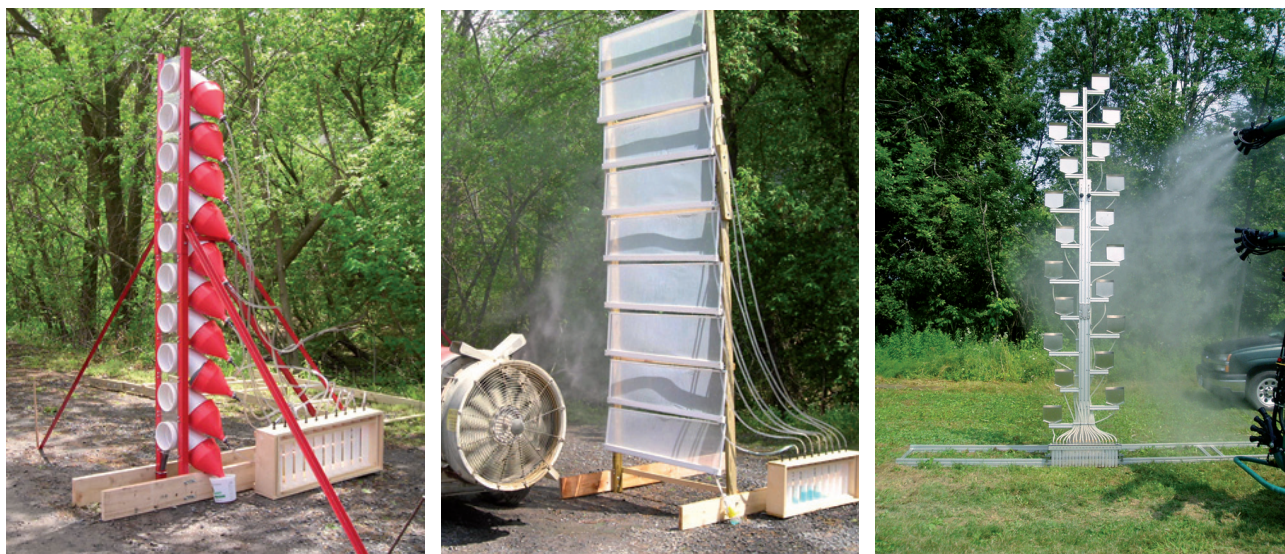
Figure 3. Three vertical patternators compared. Developed prototypes: UPC (left) and Cornell (center) were compared with MIBO commercial vertical patternator (right).
