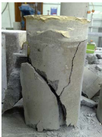
Figure 13: Failure mode of 1000 kg/m 3 density at ambient temperature
