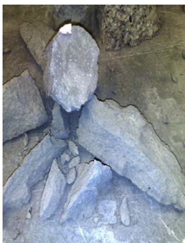
Figure 15: Failure mode of 1000 kg/m 3 density at 600°C
