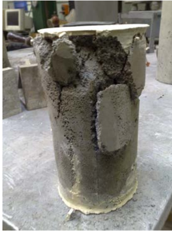
Figure 10: Failure mode of 650 kg/m 3 density at ambient temperature
