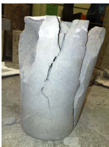
Figure 14: Failure mode of 1000 kg/m 3 density at 400°C
