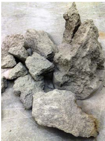
Figure 12: Failure mode of 650 kg/m 3 density at 600°C
