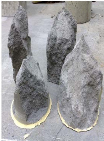
Figure 11: Failure mode of 650 kg/m 3 density at 400°C
