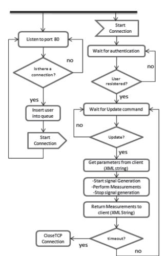
Figure 1. State Diagram of the Server.
