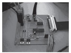
Figure 2. PCB with the ASIC.
