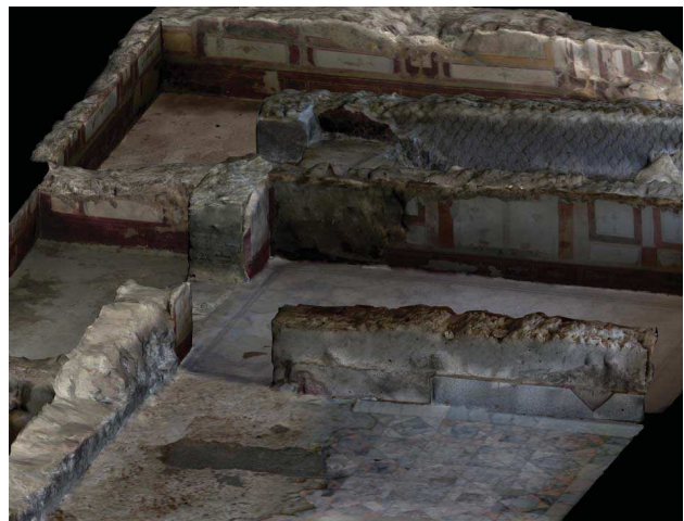
Figura 9. 3D model of the Villa of Livia by laser scanning data
