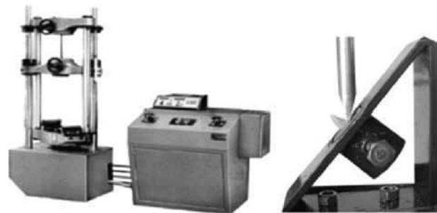
Figura 3. Maquina Universal de Pruebas, para estudios in vitro . Tomado de Evaluation of fracture resistance in simulated immature teeth using Resilon and Ribbond as root reinforcements--an in vitro study. Dent Traumatol. 2009;25:433-8
