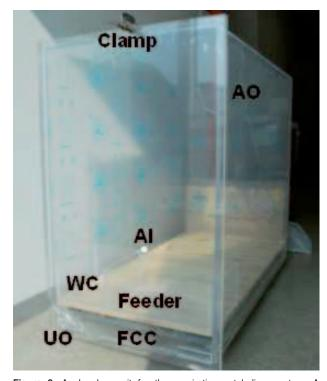
**Figure 3.** A chamber unit for the respiration-metabolism system. A chamber is made of 10-mm transparent acryl panels (1.30 m long, 1.00 m high, and 0.60 m wide for the 3 large chambers and 1.10 m long, 0.80 m high, and 0.60 m wide for the 1 small chamber demonstrated in Figure 2); Al: air inlet through a 15-mm diameter hole; AO: air outlet through a 25-mm width wood panels with 15-mm gaps between panels; FCC: fecal collection container; UO: urine outlet; WC: water cup.
