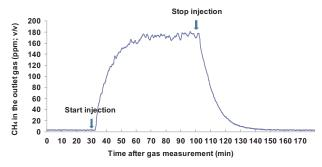
**Figure 4.** An example of methane recovery tests. The standard gas was released starting at 30 min and continued until 100 min. The basal concentration of  $CH_4$  was calculated based on the data during the first 30 min. Recovery rate (%) was calculated as the ratio of the recovered amount of  $CH_4$  gas to injected amount of  $CH_4$ .
