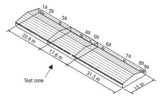
**Figure 5.** Commercial poultry building showing the experimental test zone, 56 wall inlets and 9 exhaust fans (six type «a» and three type «b»).
