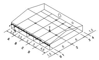
**Figure 7.** Measurement points in the test zone (distances in meters) and mobile post with sensors at three heights: 0.2 m, 0.6 m and 2 m.
