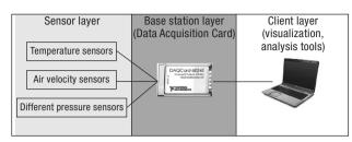
Figure 1. Diagram of system components.
