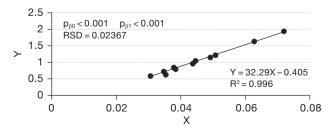
**Figure 3.** Calibration line for air velocity sensors.  $p_{\beta 1}$ : probability value for the slope.  $p_{\beta 0}$ : probability value for the intercept. RSD: residual standard deviation.
