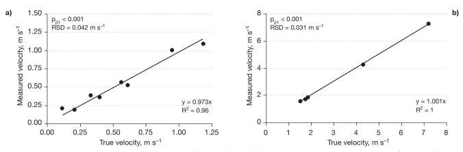
**Figure 4.** Measured and true air velocity from the calibration of one of the sensors. a) Range from 0.1 to 1.5 m s<sup>-1</sup>; b) range from 1.5 to 7 m s<sup>-1</sup>;  $p_{\beta_1}$ : probability value for the slope; RSD: residual standard deviation.
