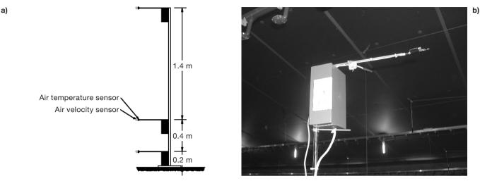
Figure 6. Measurement post showing sensors at three levels (a) and photo showing the sensors (b).
