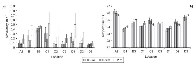
**Figure 8.** Air velocity (a) and air temperature (b) measured at nine locations of the test zone, at three heights: 0.2 m, 0.6 m and 2 m. Error bars show standard deviations.
