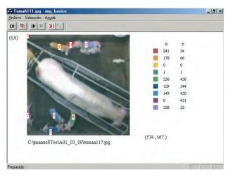
**Figure 8.** Detection error: colour 2 visible, but not detected (coordinates (0,0)).
