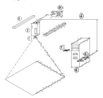
**Figure 1.** System for data capture. 0, lighting; 1, lens; 2, CCD camera; 3, feeder; 4, coaxial cable; 5, capture card; 6, PC ; 7, capture software.
