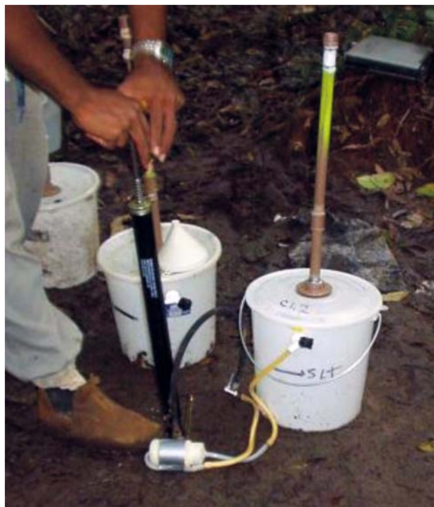
Figure 3. Photograph of flushing of CO 2 bucket chamber with CO 2 -free air prior to soda lime placement.
