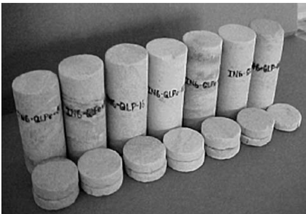
Figure 1. Unconfined compression test specimens (1"x2") and (~5mm thick) used in Indentation test
