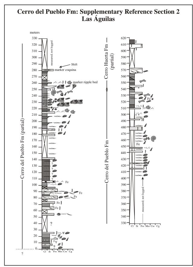
Figure 8. Measured Supplementary Reference Section (#2) at Las Águilas. All abbreviations as in Figure 5. Note the thick, non-redbeds interval.
