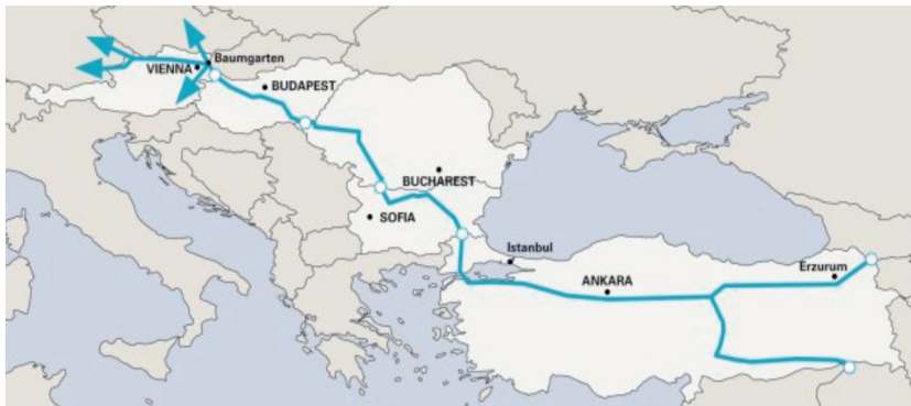
Figure 4.5. Nabucco Gas Pipeline (would join up with the BTE in Erzurum)
