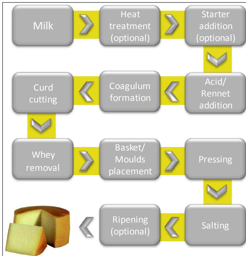
**Figure 1.** Flow diagram for general cheese production (adapted from Bonet et al. 2009).
