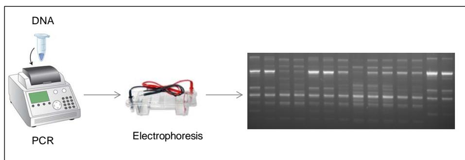
**Figure 7.** Flow diagram of RAPD analysis.
