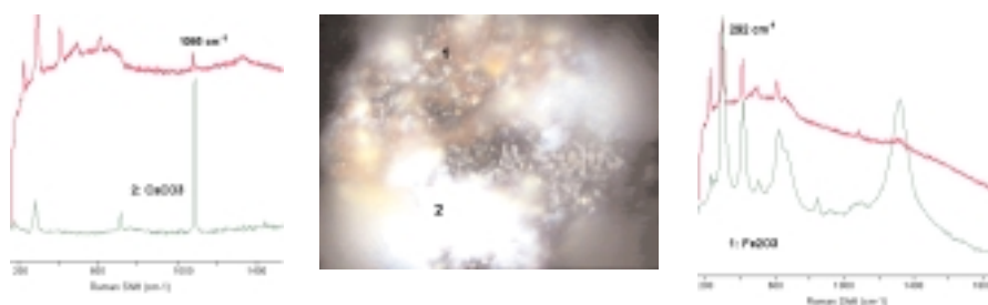
Figure 2. Micrograph of a small piece of glass and Raman Spectra recorded across the glass surface (in red). Components were identified by comparing with Renishaw Raman Library.
