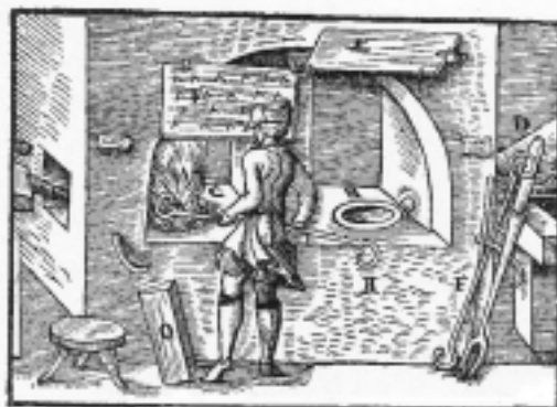
Figure 1. Refining silver in a cupellation hearth (from Ercker 1574).
