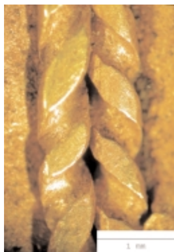
Figure 3. Photograph, in unpolarized light, of the simulated wire braiding on the filigree. The edges display that this is twisted flat strip.
