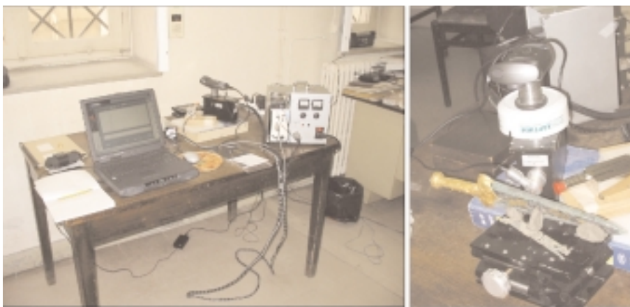
Figure 2. The instrumentation set-up during the measurement of the Dagger 8340.
