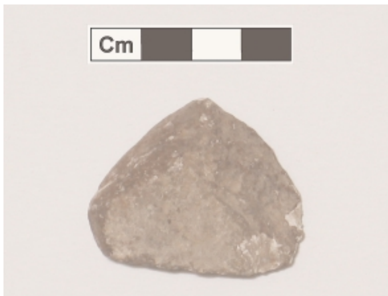
Figure 4. Litharge impregnated hearth lining fragment from Daskaleio-Kavos.
