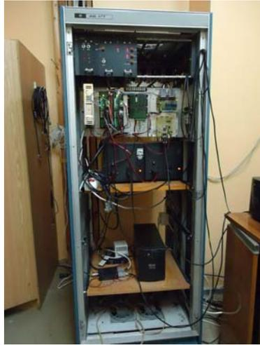
Figure 17. The control panel. From top to bottom: power supply; JVL driver SMC 35 SMD41B3 (green color); GPS Garmin 35 LP.
