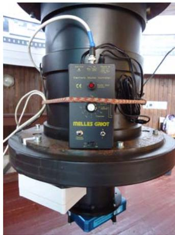
Figure 19. Electronic Shutter Melles Griot 43 mm.
