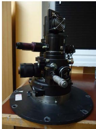
Figure 7. Three-channel high Speed CCD photometer.
