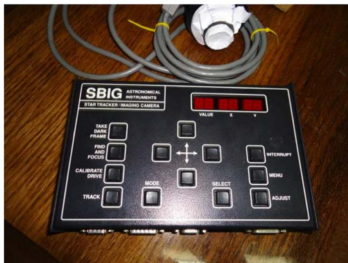
Figure 23. Star Tracker/Imaging camera. "Santa Barbara Instrument Group" (SBIG) CCD camera autoguider
