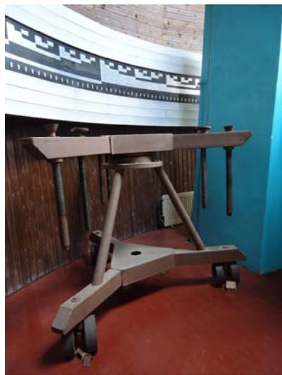
Fig. 12. Cleaning table for the mirror of 1.65 m.
