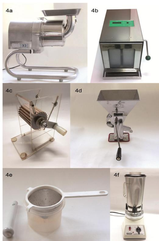
Fig. 4: Illustration of the different materials tested for grape juice extraction: a) ASieves, b) BMixer, c) Crusher, d) TPress, e) Manual and f) Blender.
