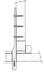
Figure 12 Palladio's *arpice* interpreted by Gennaro Tampone; perspective drawing made by Pictro Copani
