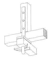
Figure 13 Palladio's *arpice* interpreted by Gennaro Tampone; perspective drawing made by Pietro Copani
