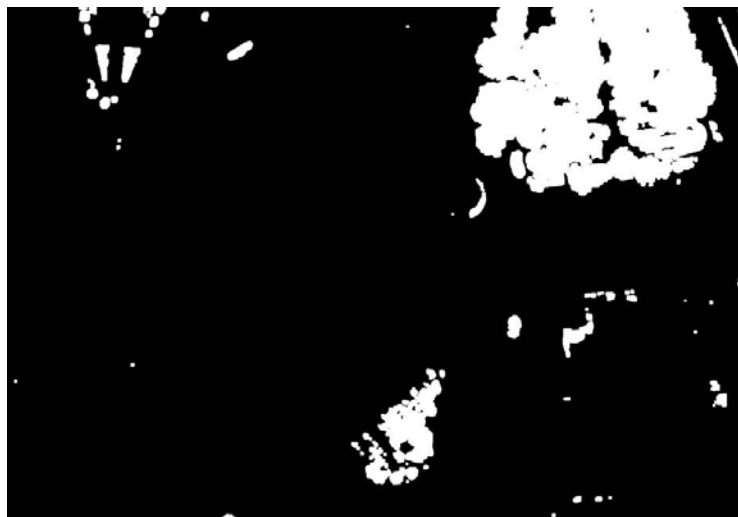
Illustration 2: Output image after merging IRG and RGB images for the process of detection of green areas.
