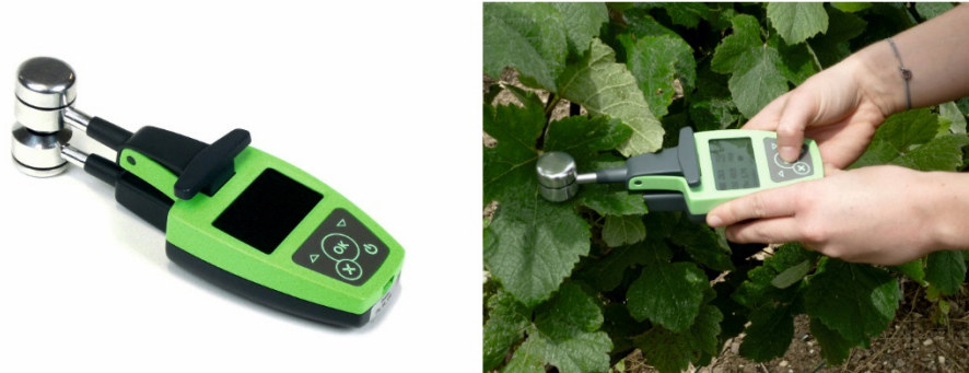
Figure 16. Optical sensor Dualex4™ (left) and an example of the measurement of a grapevine leaf (right) (Force-A).
