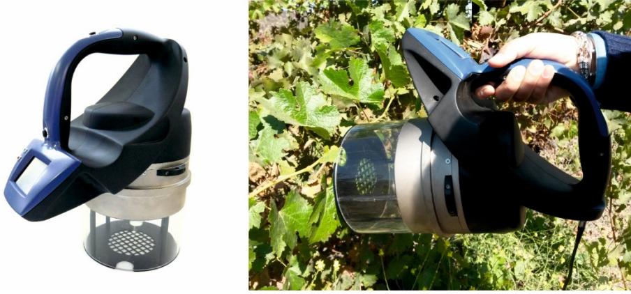
Figure 17. Fluorescence sensor Multiplex™ (left) and an example of the measurement of a grapevine leaf (right) (Force-A).
