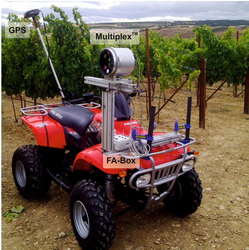
Figure 30. The three components of the fluorescence sensor mounted on a quad: Multiplex™ sensor, FA-BOX and GPS (Force-A).
