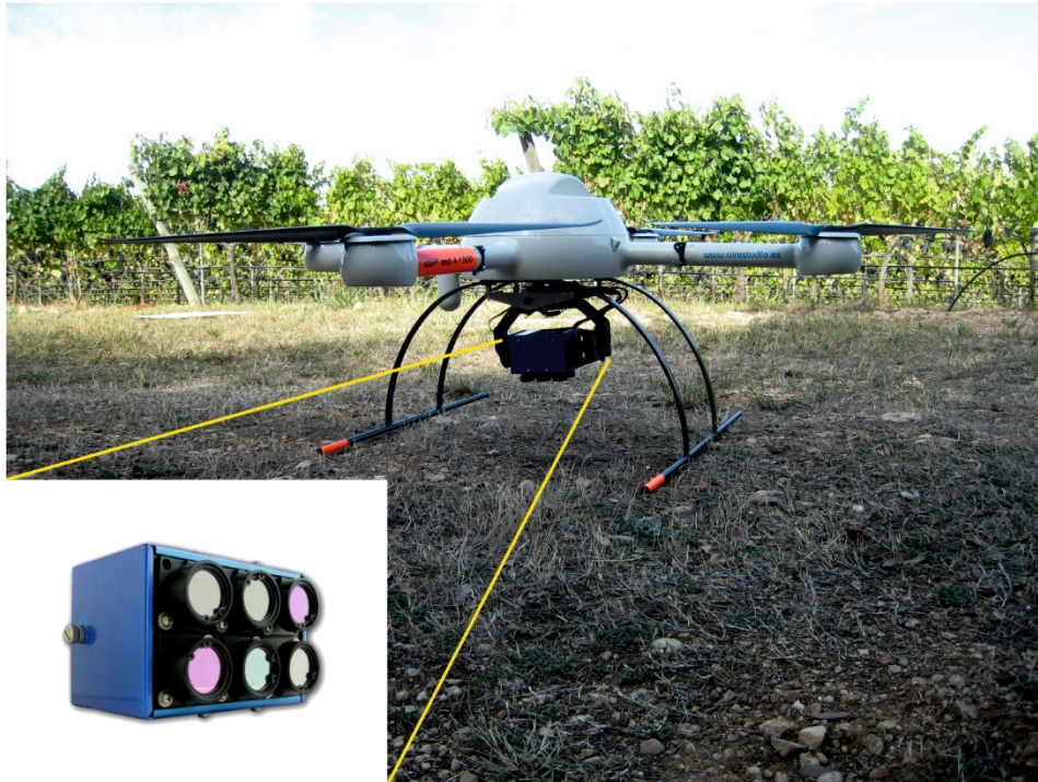
Figure 11. Multispectral camera mounted on the RPAS Md4-1000 and detail of the multiple camera array.
