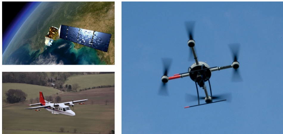
Figure 4. Different platforms in remote sensing. On top-left, the Landsat 8 satellite (NASA); bottom-left, an airborne platform (NERC); and on the right, a remotely piloted aerial system (RPAS).
