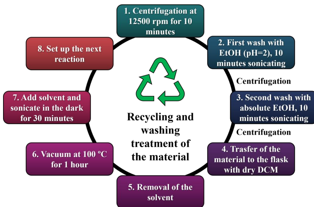
Figure 2.18. Schematic representation of the photocatalyst washing process in each of the catalytic cycle for the synthesis of phenanthridine.
