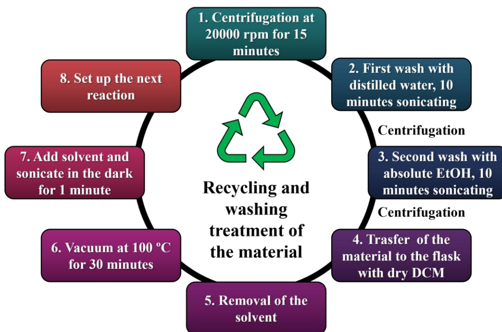
Figure 2.14. Schematic representation of the photocatalyst recovery and washing process in each of the catalytic cycle for the dehalogenation reaction.
