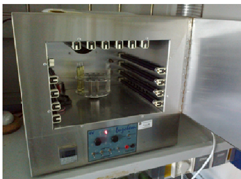
Figure 5.35. Image of the photoreactor used for irradiating under these conditions.
