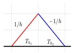
Figure 2. Derivative of the shape functions on the intervals  $\frac{d\varphi_i}{dx} = \frac{1}{h}, \frac{d\varphi_{i+1}}{dx} = -\frac{1}{h}$  [17].
