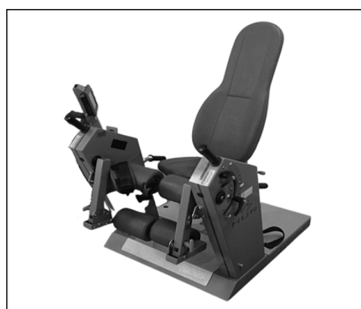
Figure 1. Leg Extension/Curl Rehab exercise machine with pneumatic resistance (HUR® 5530) used for the isometric muscle strength measurements.
