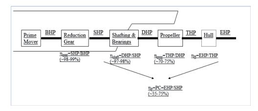
Fig. 6. Propulsive efficiency.
