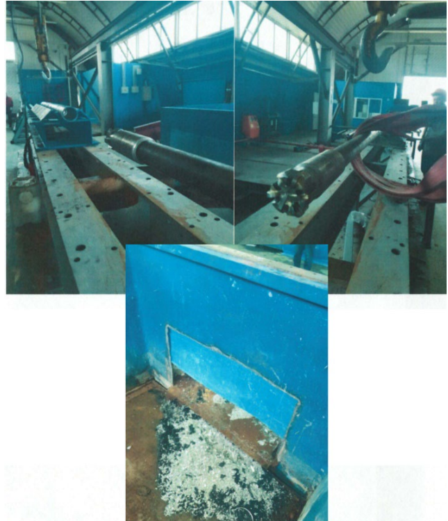
Figure 6. Drilling parameters for the BittFrac module. The drilling was rotary and tool speed was 60 \pm 2 rpm. The axial force on the tool was 0.5-1 tf, and the duration of drilling was 2 hours and 40 minutes.
