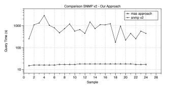
Figure 4. Time reduction; our approach (software agent approach) vs. the traditional mode (SNMP v2). Source: Authors
