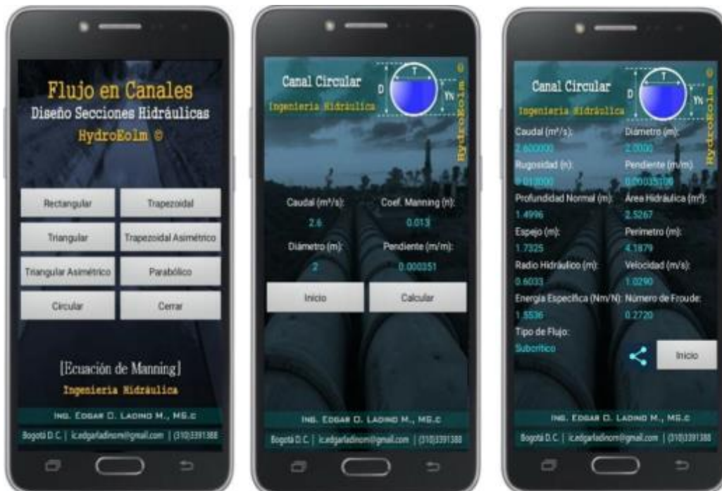
Figure 14. Exercise 2.7, Hidráulica de canales, Gilberto Sotelo (app’s normal depth calculation)
