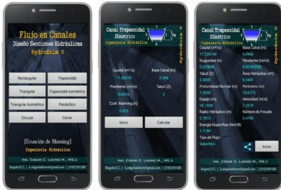
Figure 15. Exercise 6.2, Hidráulica de canales abiertos, Ven Te Chow (app's normal depth calculation)
