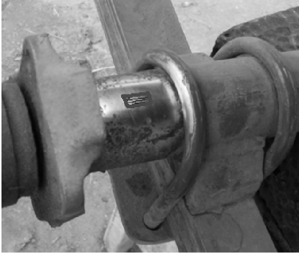
Figure 9. Strain gauge on the shaft of a spring suspension vehicle
