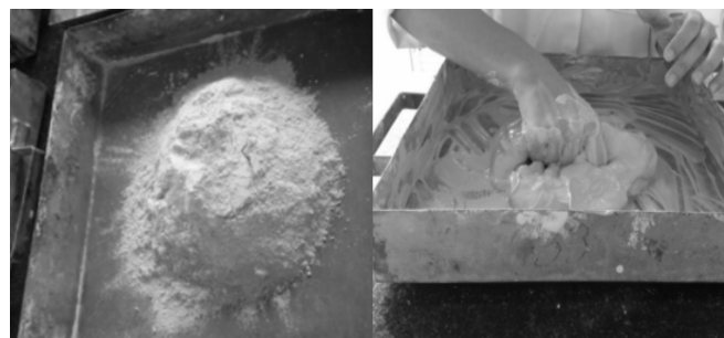
Figure 1. Sample preparation procedure: making the Kaolin clay slurry at 1.5 times the liquid limit. Left) Dried Kaolin powder. Right) Kaolin clay slurry after its hydration.
