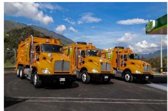
Figure 1. Vehicles run on Natural Gas solid waste collection trucks of EMVARIAS of Medellín. Source: EPM
