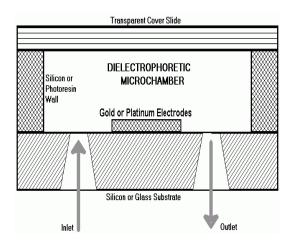
**Figure 1.** Cross section view of the proposed microdevice. In this sketch three main components may be identified: the substrate where electrodes are grown, the electrodes itself responsible for the electric field profiles, and the silicon or photoresin walls limiting the microchamber working area. A cover slide is placed on the top of the structure to close the cavity
