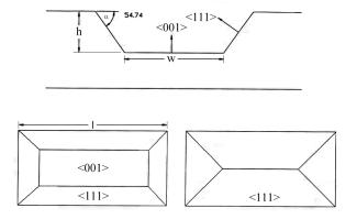
Figure 10. Cross section and top views of rectangular windows anisotropically etched on a silicon wafer aligned to direction <110>. If the window length, *l*, is small and the wafer thickness is big enough, the etching progress ends up when the four planes <111> intersect among them (rectangle on the right). However, under the adequate relationship between window area and wafer thickness, a square or rectangular hole can be drilled. (rectangle on the left) [50]
