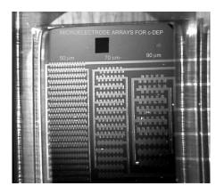
Figure 4. Platinum microstructures containing classical and shifted interdigitated castellated, as well as saw-teeth microelectrodes
