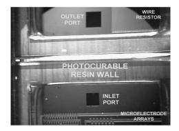
Figure 12. Partial view of the photosensitive resin walls of two adjacent chips before of being diced. Inlet and outlet ports can also be seen
