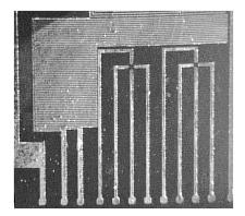
Figure 9. View of the platinum meandering wire. The assessed resistor value was 6895  $\Omega$  while its measured value was 6800  $\Omega$  at 25 °C
