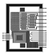
Figure 2. Mask diagram including the three required layers to process the microchip. The two red-square regions have a side length of 900 (top) and 1000 (bottom) μm and serve to build the inlet and outlet holes by micromachining. The green rectangle of 800 μm in width will be used to pattern the photoresin. The blue level contains diverse electrode microarrays and will outline the metal layer
