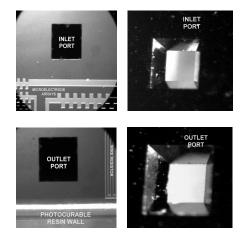
Figure 11. Front side (left) and backside (right) of the silicon substrate after anisotropic etching by means of TMAH
