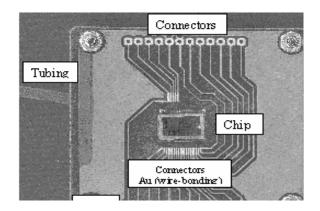
**Figure 14.** Photograph of the microsystem mounted on a PCB (5.5 cm in width and length) with wiretracks metallised of gold to facilitate the chip wirebonding procedure. Plastic tubing conveniently glued to the backside of the microstructure can be easily seen
