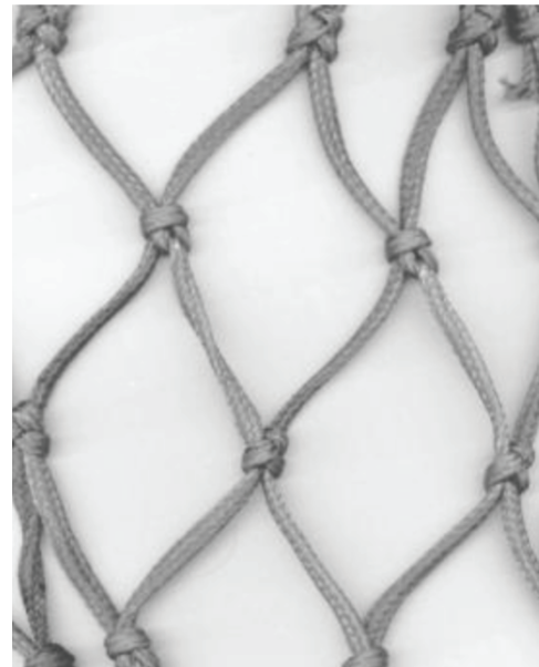
Fig. 1. Weave of a polyethylene net
