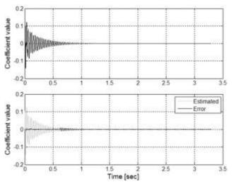
**Figure 6.** Secondary path Impulse response identification. **Source:** authors.
