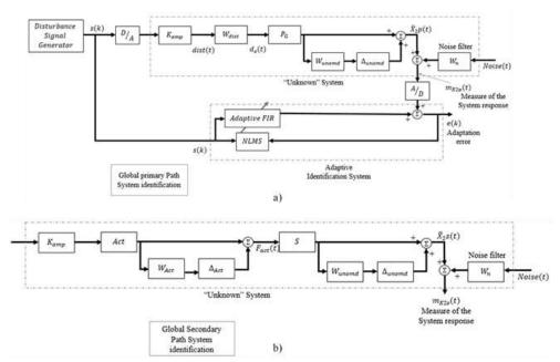
Figure 4. Secondary path Identification Using the NLMS Adaptive Filter. Source: authors.
