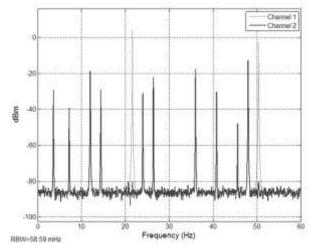
**Figure 14.** Power spectral of the AVC system using feedback FxLMS. **Source:** authors.
