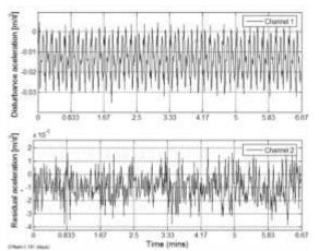
**Figure 11.** Disturbance rejection of the AVC using RLS algorithm with feedback coupling. **Source:** authors.
