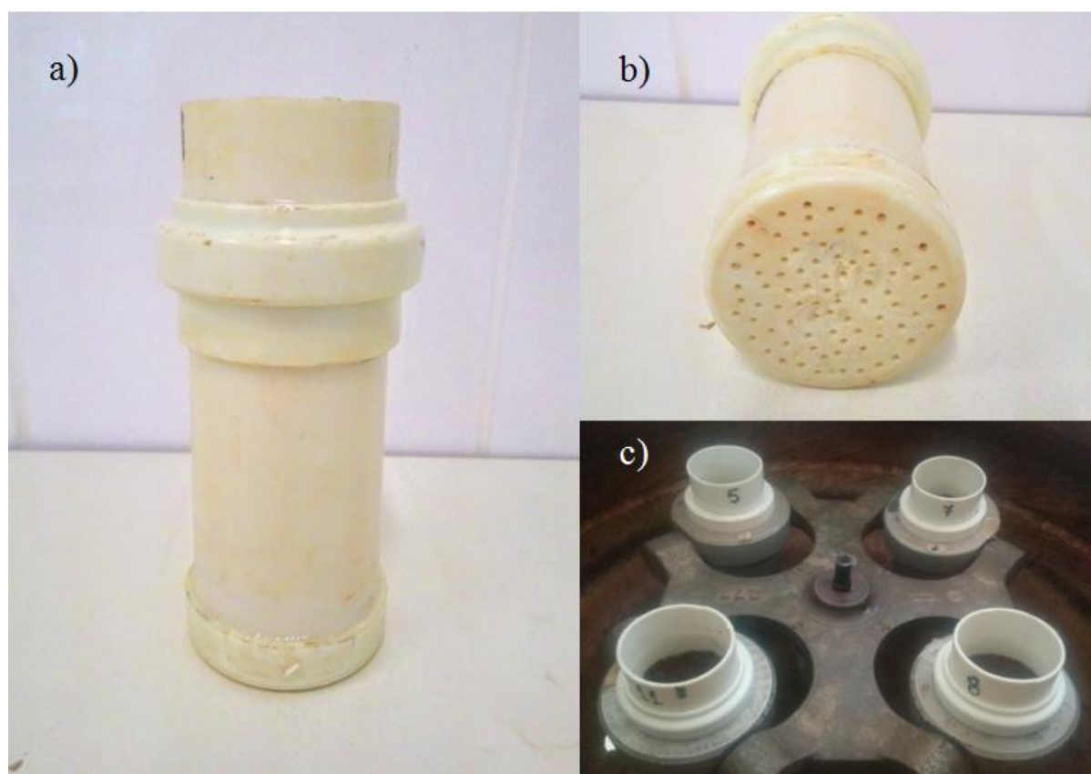
Figure 1 – a) Soil storage container. b) Perforations for soil solution extraction. c) Arrangement of samples for centrifugation process.
