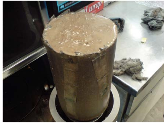
(f) Compacted sample at high molding water content
