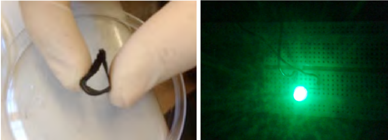
Figure 6. Flexible cotton-based SC prototype (left) and LED powered by three cotton-based prototypes connected in series (right).
