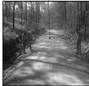
Figure 3. Dimensions, design, and road surface measurements using the rill meter.
