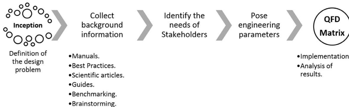
Figure 7 Diagram of QFD generation
