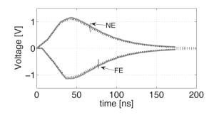
**Figure 4.** Voltages on the Victim Wire at the Near and Far End (Solid Line: FDTD uniform orthogonal mesh, Dashed Line: FDTD non-uniform orthogonal mesh).
