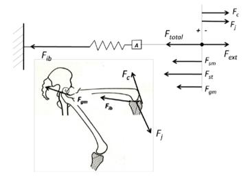
FIGURE 1: Forces applied in the shank during knee extension.
