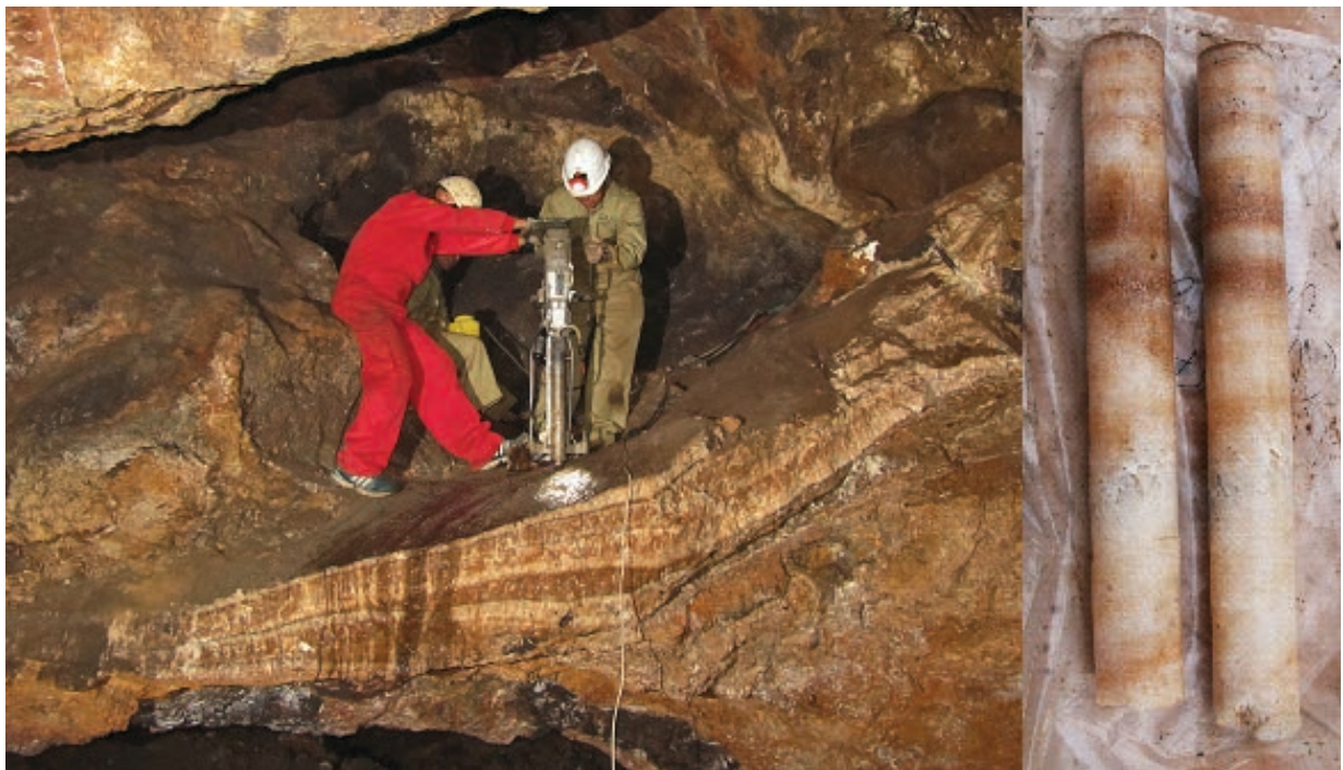
Fig. 2. (Left panel) Sampling of the Cueva Victoria flowstone sequence using a mobile drilling machine (picture courtesy of C. Rossi). (Right panel) The obtained cores have a length of ca. 50 cm and a width of 5 cm.
