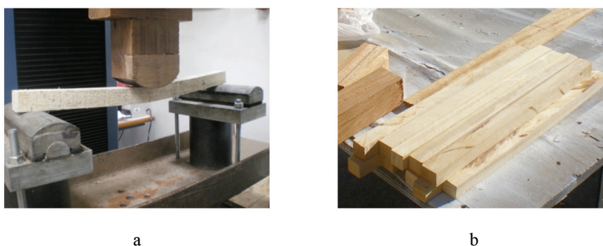
Figure 12. a. Static bending test assembly showing load application and specimen support. b. Brosimum utile specimens.
