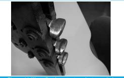
Figure 11 Worn fixed contacts selector switch
