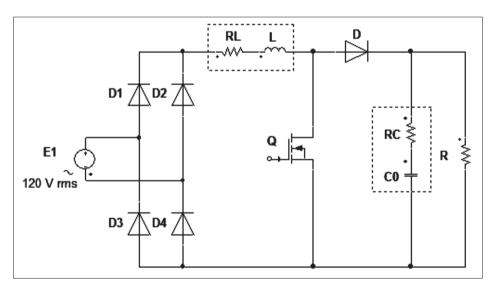
Figure 1. The DC/DC boost converter. This switching-mode converter contain two semiconductor switches (Q and D) and one energy storage element (L). The output capacitor (Co) works as filter. Source: Own source.
