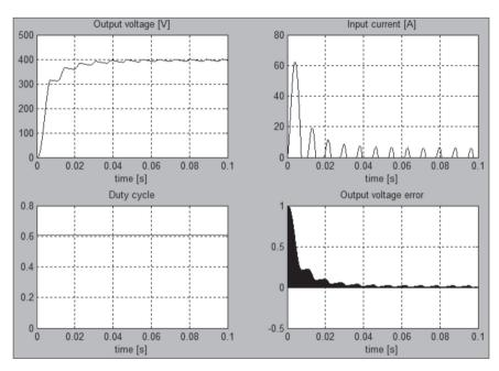
Figure 2. Step response of boost converter (simulation open loop). Starting current greater to 60 A. Source: Own source.
