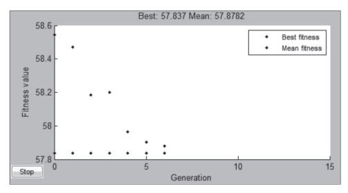
**Figure 4.** Convergence of the GA algorithm (one hour and 55 minutes of simulation in a AMD Athlon 64 3200+). Source: Own source.
