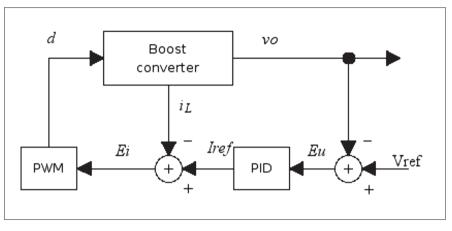
Figure 3. Control system configuration of research target. Two loops control, one in voltage mode and another in current mode are used.
