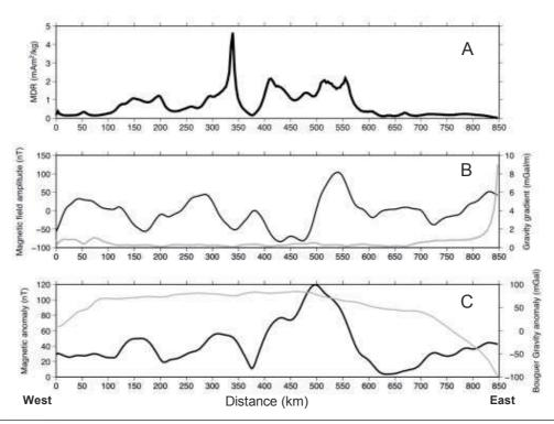
FIGURE 3 MDR profile (see Figure 2 for location). A) MDR values. B) Magnetic field amplitudes (black line) and gravity gradients (grey line), in nT and mGal/km, respectively. C) Magnetic anomaly (black line) and Bouguer gravity anomaly (grey line), in nT and mGal, respectively. Both gravity and magnetic data were upwardly continued to 10 km above sea level (see text for comments).
