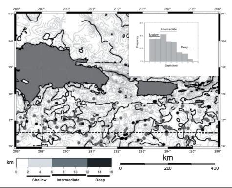
FIGURE 4 Euler solutions overlying the contour scalar magnetic map for a structural index (SI) of 2.5 and a depth tolerance of 15%. Inserted histogram with a depth estimation of the centroid's causative body location (see text for comments). Contour interval: 50nT. The isoline 0nT is plotted in black. The black dashed line traces the MDR profile of Figure 3 (this profile is modeled in Fig. 5). SPB: San Pedro Basin.
