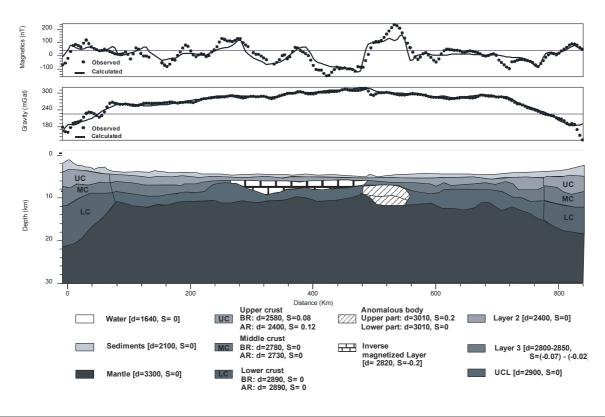
FIGURE 5 Magnetic and gravity models for the east-west profile. Magnetic units: nT. Gravity units: mGal. Susceptibility units: S.I.. Density units: kg/m<sup>3</sup>. Profile location is shown in Figure 2. BR: Beata Ridge. AR: Aves Ridge. UC: Upper crust. MC: Middle crust. LC: Lower crust. UCL: Underplate Cumulate Layer.
